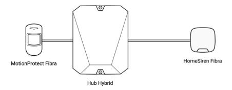
MotionProtect Fibra is a wired motion detector. Using IR sensors, the detector can identify intrusions by detecting moving objects with temperatures close to the human body.
